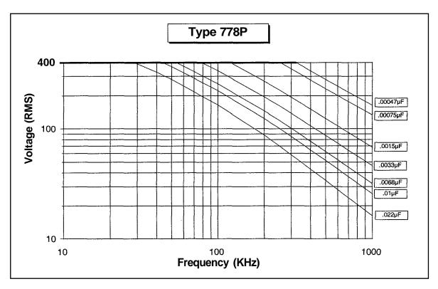
RMS Voltage vs. Frequency @ +85°C
