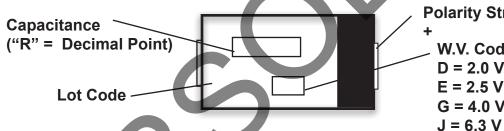
Polarity Stripe (Anode) + W.V. Code D = 2.0 V K = 8.0 V E = 2.5 V B = 12.5 V G = 4.0 V C = 16.0 V
