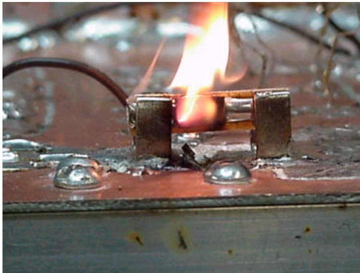
Fig. 6 Two minute Exposure of 33 \mu F, 10 V Tantalum Capacitor to 10 V, 1 kHz Squarewave
