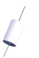
Type 935 metallized polypropylene capacitors are designed for filtering applications in switching power supplies that operate in the 20-100 kHz range. Their low ESR, high current and high capacitance gives them an advantage over general purpose types. This series is UL recognized for construction only under UL File Number E128034(N).
