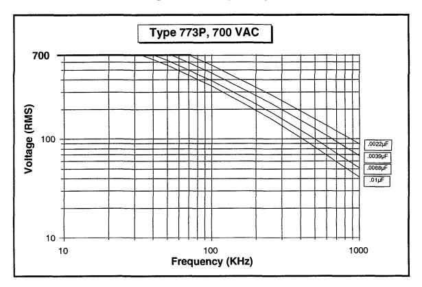
RMS Voltage vs. Frequency @ +85°C
