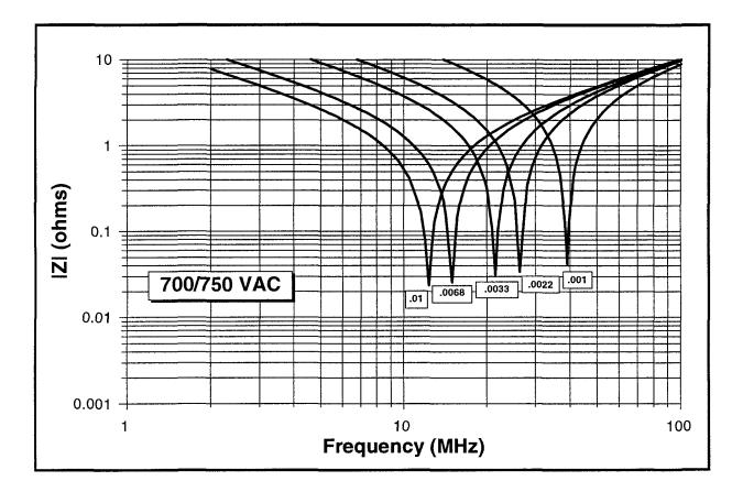
Please note: Capacitance values above are in  $\mu$ F. The resonant frequency and impedance shown above apply to units with a 0.250" lead length and are typical values only. Please contact us for additional data.
