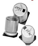
Type AEB capacitors are it for high voltage applications like input bus capacitors in board mounted miniature AC/DC supplies. The AEB's low impedance in ratings up to 450 Vdc, and long life, make it ideal for power supply input and other high voltage applications. The vertical, cylindrical cases make easy automatic mounting and reflow soldering.
