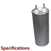
Type PC capacitors are designed to meet the demands of filter applications rich in system total harmonic distortion (THD). This series has a dual protection system utilizing self healing metallized polypropylene and a mechanical pressure interrupter to ensure a safe open circuit mode in the event of overload or end of life. (\*)
