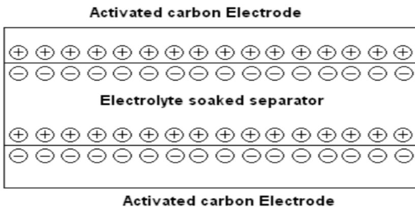
The double layers formed on the activated carbon surfaces can be illustrated as a series of parallel RC circuits.
