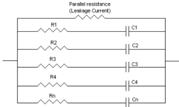
When voltage is applied current flows through each of the RC circuits. The amount of time required to charge the capacitor is dependant on the CxR values of each RC circuit. Obviously the larger the CxR the longer it will take to charge the capacitor. The amount of current needed to charge the capacitor is determined by the following equation:
