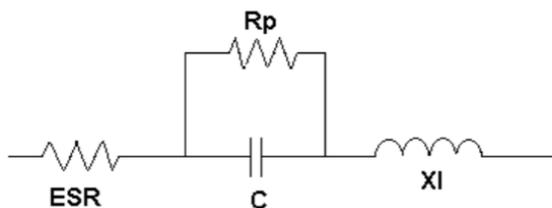
This equivalent circuit is only a simplified or first order model of a supercapacitor. In reality supercapacitors exhibit a non-ideal behavior due to the porous materials used to make the electrodes. This causes supercapacitors to exhibit behavior more closely to transmission lines than capacitors. Below is a more accurate illustration of the equivalent circuit for a supercapacitor.
