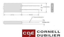
This mechanical drawing of a THA Series device highlights dimensional characteristics., nominal lead lengths and 20 gauge size.
