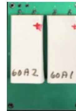
Prismatic Aluminum Electrolytic Bank 95\mu\text{F} @ 500\text{ Vdc} , 150^\circ\text{C}
