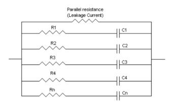
When voltage is applied current flows through each of the RC circuits. The amount of time required to charge the capacitor is dependent on the CxR values of each RC circuit. Obviously the larger the CxR the longer it will take to charge the capacitor. The amount of current needed to charge the capacitor is determined by the following equation:
