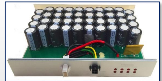
High-Voltage, High-Capacity Custom Module Example
