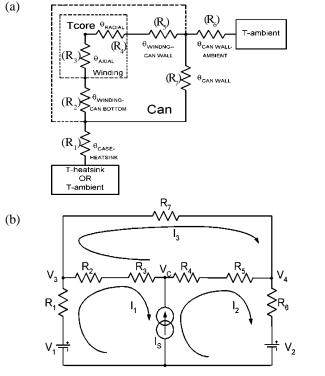
Fig. 2. (a,top) Thermal circuit equivalent for bus capacitor; (b,bottom) electrical circuit analogy.
