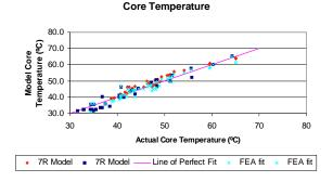
Fig. 7. Comparison of results from the 7R lumpedparameter thermal model and FEA-equation solver model versus test data. The test data includes capacitors in still air, isothermal heat sink, and moving air from 80 to 1000 LFM. Core rise above ambient was generally 10 - 30 °C. Capacitor sizes range from 1.375" diameter to 3.0" diameter.
