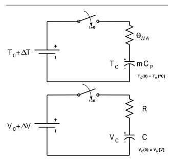
Fig. 5. (a,top) Transient thermal circuit equivalent for bus capacitor; (b,bottom) electrical circuit analogy.
