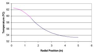
Fig. 4. Graph of the radial temperature distributon of a circular aluminum chassis plate with a center mounted capacitor.
